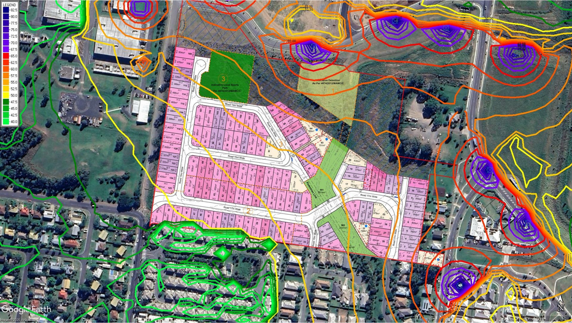
Plate B4: Industry noise contours at 4.6m (first floor height). Levels are in dB(A) L10 and are façade-adjusted.
