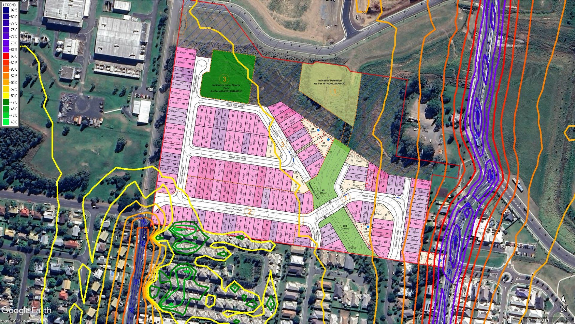
Plate B2: Road traffic noise contours at 4.6m (first floor height). Levels are in dB(A) L10,18hr and are façade-adjusted.
