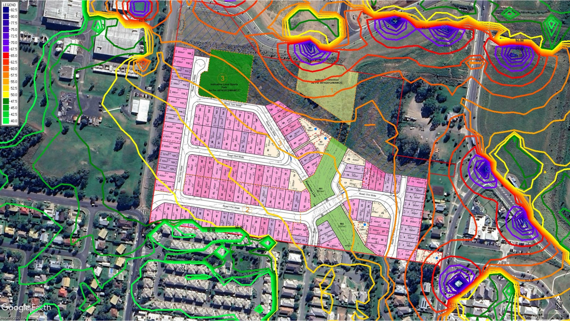
Plate B3: Industry noise contours at 1.8m (ground floor height). Levels are in dB(A) L10 and are façade-adjusted.
